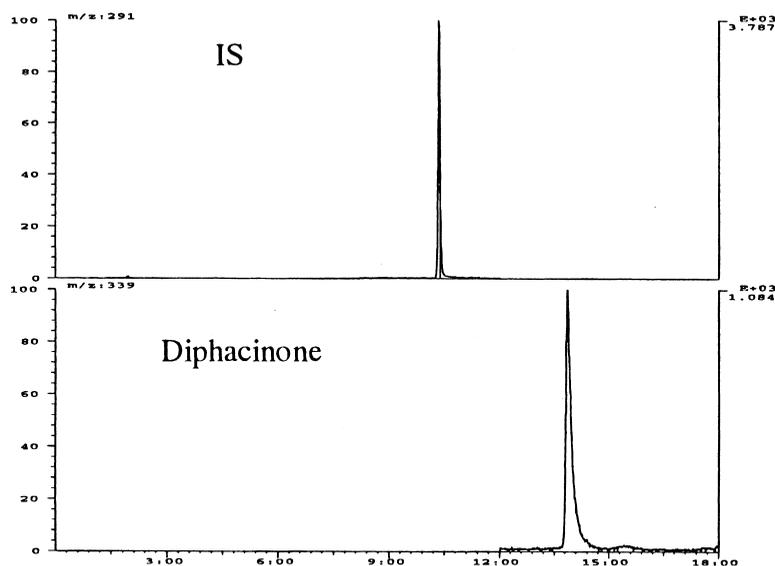
Fig. 6. Time-scheduled SIM chromatograms for a blood sample from a rat dosed with 50 µg of diphacinone. The blood sample was taken 3.5 h after administration, and 500 ng of coumatetralyl (IS) was added to 1 ml of the blood sample prior to liquid–liquid extraction. The left and right vertical axes and the horizontal axes are the same as those in Fig. 4. For other conditions, see the Experimental section.
