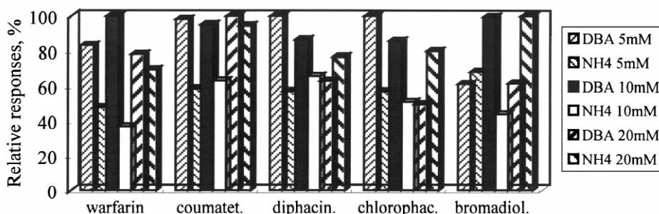
Fig. 3. Comparison of DBA and ammonium acetate (AA) buffers for MS responses of anticoagulant rodenticides. Each analyte was injected into the flow of mobile phases containing different concentrations of DBA and ammonium acetate separately (direct flow method), which entered APCI–MS directly, monitored by SIM, and the peak heights were averaged for six repeated injections. For other conditions, see Fig. 2.
